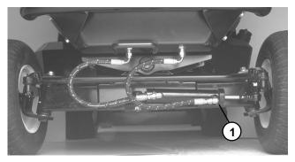
Figure 18 1. Right side steering cylinder fitting
